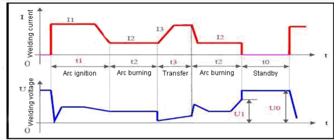
Current and Voltage Changes in DC MMA
