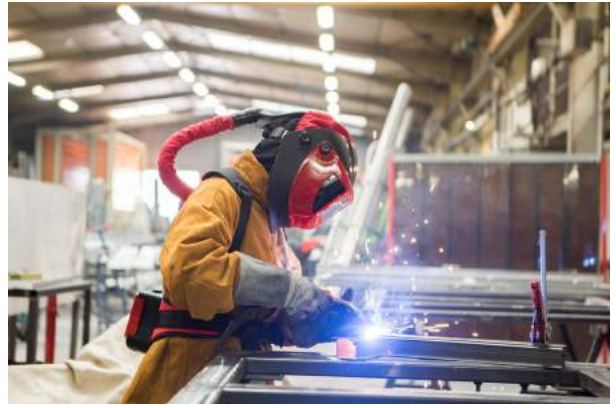
An example of personal fume extraction
