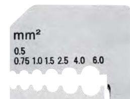
12 21 180: wire cross-sections in mm 2
