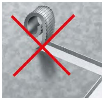
Notching without chip breaking
