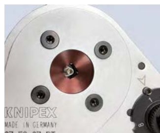
Synchronous feed of the four mandrels achieves optimum crimping results with eight indentations (4/8-Indent)
