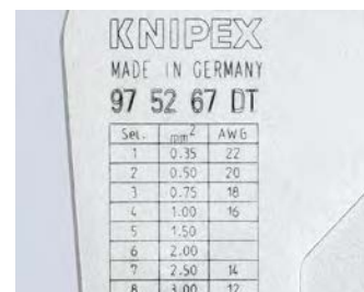
Selector positions for setting the crimp depth can be clearly read on the pliers
