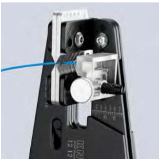
Precise cutting of the insulation to a complete extent
