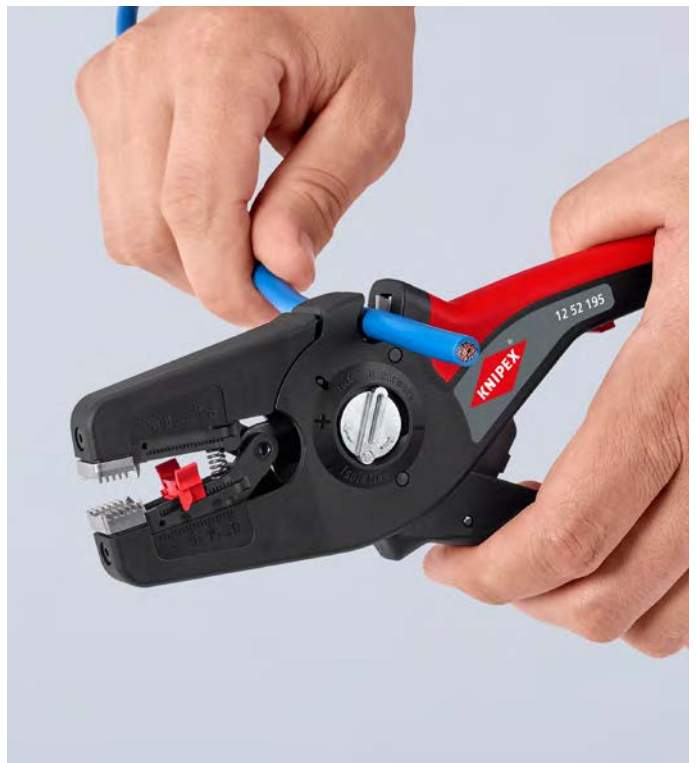
With cable cutter on top for copper and aluminum conductors, flexible up to 16 mm 2 (AWG 6), solid up to 6 mm 2 (AWG 10)
