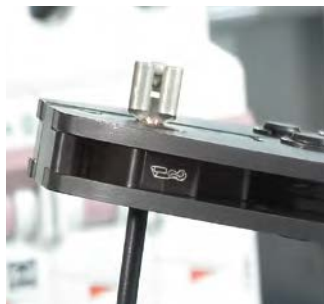
Clearly visible marking on the crimping dies with pictograms
