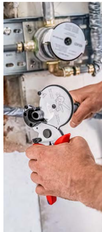
The pipe cutter cuts all common composite and plastic conduit pipes with diameters of up to 26 millimetres. Its robust construction means it is also suitable for composite conduit pipes with increased aluminium layer thickness
