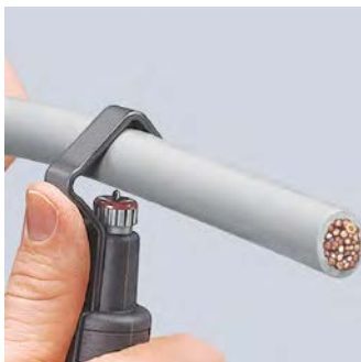
Setting the tool for circular cut
