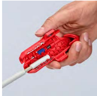
Stripping of a NYM cable
