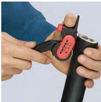
Setting the tool for longitudinal cut
