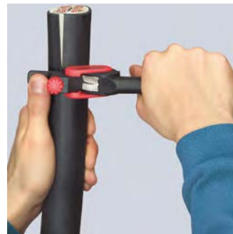
Turning the tool for circumferential cut
