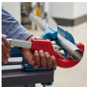
For cutting copper, brass and stainless steel pipes and rigid steel conduits with wall thickness up to 2 mm and diameters of 6–35 mm (1/4–1 3/8")
