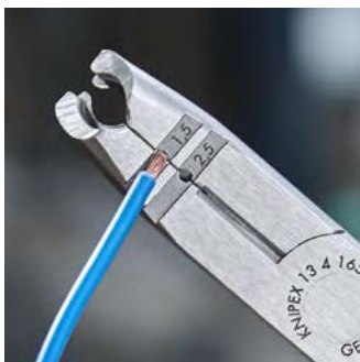
Wire stripping holes for 1.5 and 2.5 mm 2 conductors
