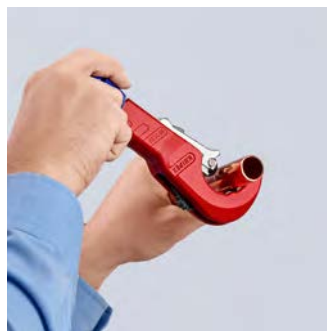
Tighten and cut with a swift twist and then readjust using the ergonomic blue feeding barrel...
