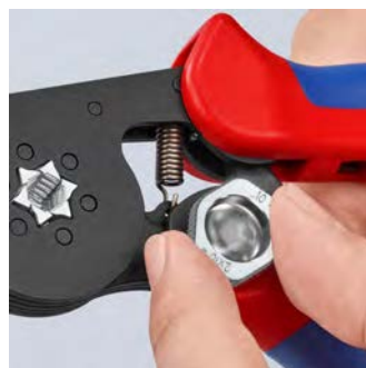
97 53 14 / 97 55 14: the crimping pliers can be adjusted to large wire ferrules of 16 mm 2 or 2 x 10 mm 2 with the adjusting wheel
